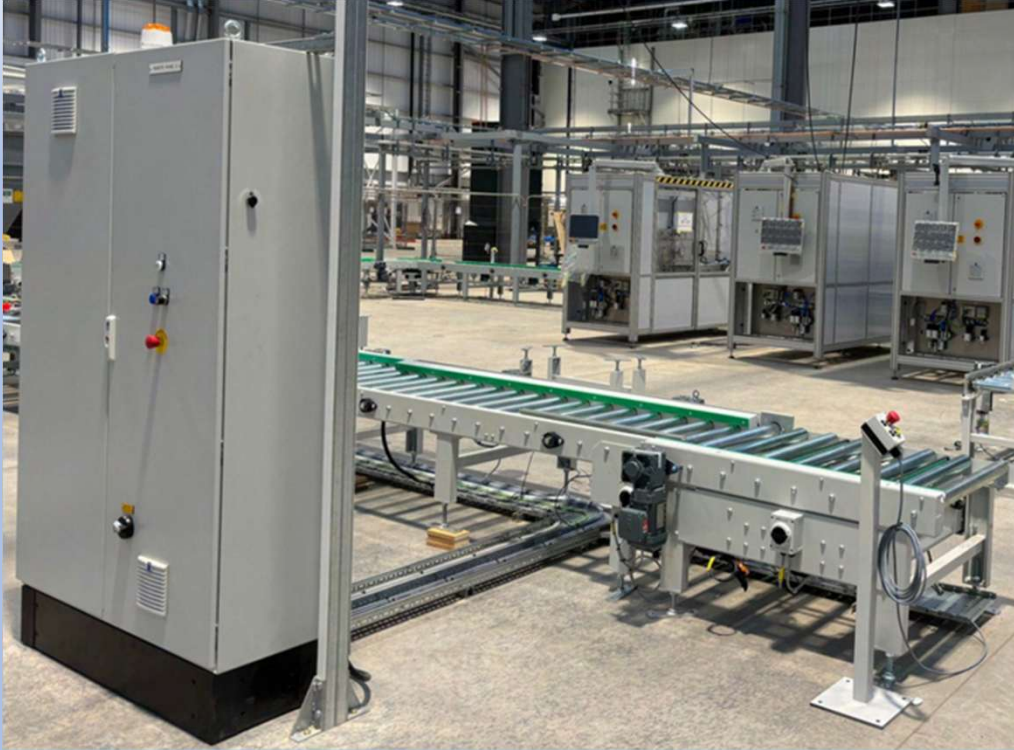
Conveyor Panels with servo and VFD controls provided with PLC programming
